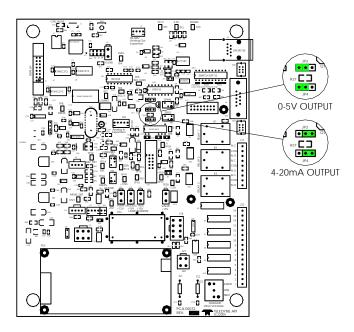
Figure 9-4: Mainboard – Analog Output Configuration
